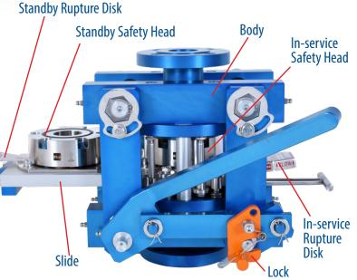
Above: Saf-T-Change<sup> $\dagger$ </sup> wetted parts include body, rupture disk, and rupture disk safety head. Standby disk and safety head is protected by a cover (not shown above).
