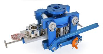
Above outlet view of a 1.5" (40mm) Saf-T-Change™ quick disk replacement. A lever or gear box is used to spread the half bodies by 5/32" (4mm). The slide is then moved to position the standby rupture disk. Only one operator is required to complete the task
